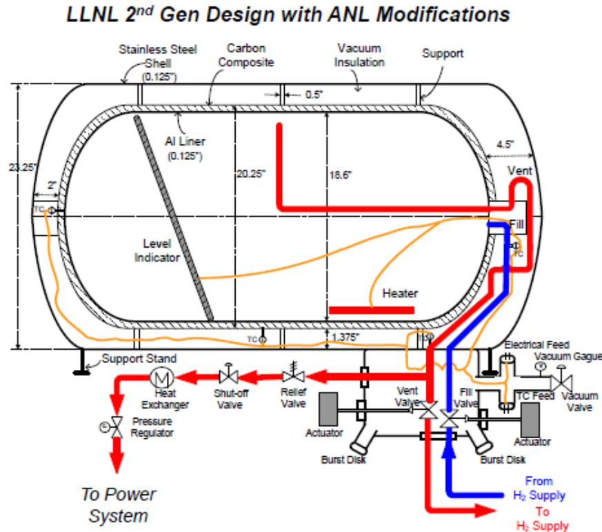
Cryo-Compressed Hydrogen Storage System Schematic<sup>1, 2</sup>
