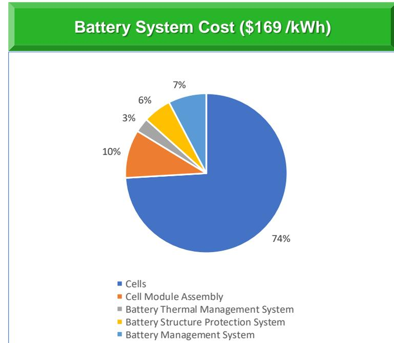
The 16 kWh lithium-ion battery system costs \$2,700 per pack at the annual production volume of 10,000 packs.
