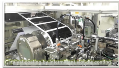
Example: Current Toyota fuel cell electrode coating
