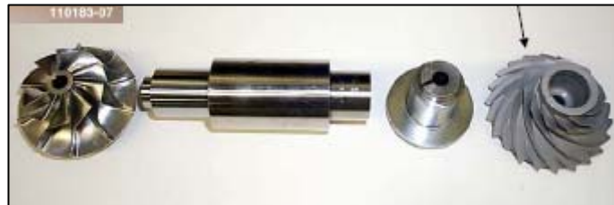
Turbine, Compressor, Shaft: Honeywell, DOE Merit Review, 2003
